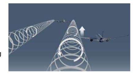
New specific & automated control laws & sensors to optimize and maintain the position within the vortex
